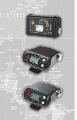
Sensitivity for  $^{137}\text{Cs: }100~\text{cps/(}\mu\text{Sv/h)}$  or better γ - channel energy range: 0.033 - 3.0 MeV Neutron channel energy range: thermal - 14 MeV (for PM1401GNA/GNM, PM1703GNA/GNM) Dose rate range: 0.01 - 99.99 µSv/h
