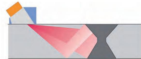
For one phased array probe, multi groups of element and multi angles can be applied for scanning at the same time, fully covering the welding area and enhancing the inspection efficiency.
