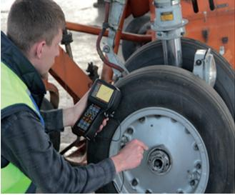
**Set of eddy current equipment for non-destructive testing of aircraft parts on the basis of "EDDYCON C" flaw detector is used for detection of surface cracks in various parts, cracks in holes and multilayered structures, surface and subsurface corrosion. Eddy current is an acceptable method for detecting conductivity of non-ferrous materials and paint thickness.**
